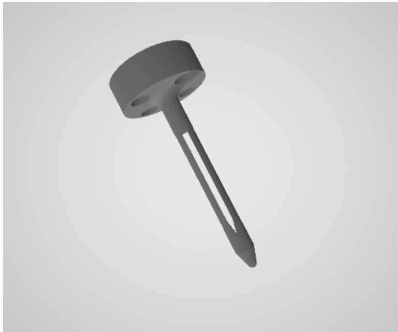
Figure 7.8: 3D version of the TCP pointer.
